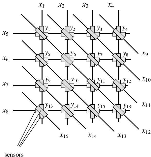
Fig.1. Architecture of the distributed measuring network with configuration  $4 \times 4$ .
