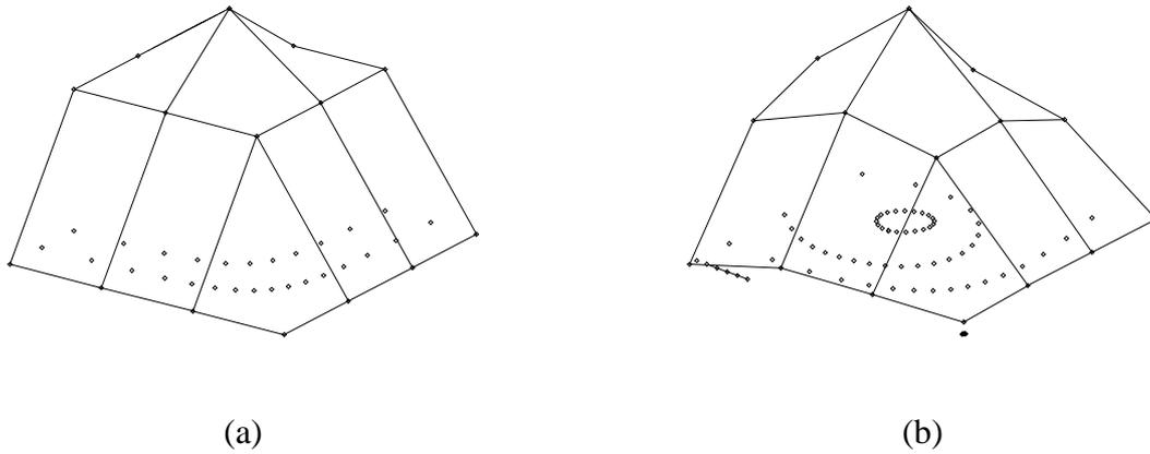
Fig. 5. The original (a) and reconstructed by the neural network (b) unknown acoustic field distribution. The original distribution was detected with the mock-up of the interferometric fiber-optic measuring system [6].
